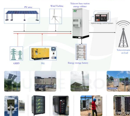
Base station energy composition diagram
