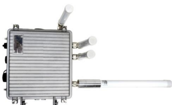
LoRawan outdoor base station
