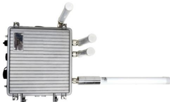
LoRawan outdoor base station
