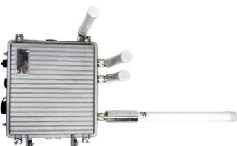
LoRawan outdoor base station
