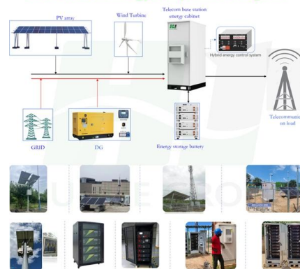
Base station energy composition diagram
