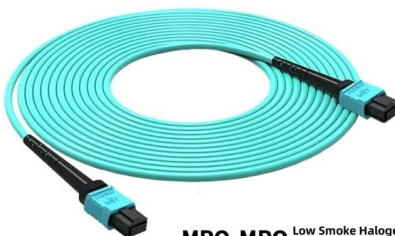
MPO-MPO Low Smoke Halogen Free Sheath Multimode 10 Gigabit 24 pole OM3 Insertion loss <0.35dB Return loss >50dB
